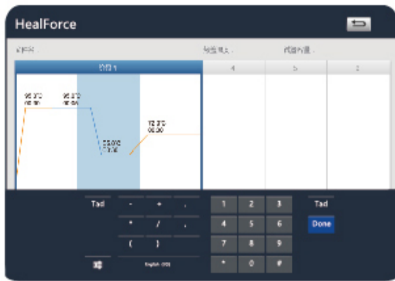
The temperature change rate can be set in a single section to meet demanding experimental requirements.
